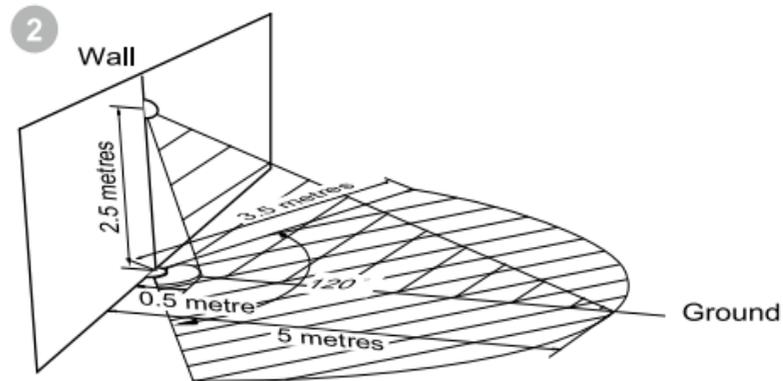
For optimal performance, your MultiSensor should NOT be mounted directly on or near metal framing or other large metallic objects. Large metal objects may weaken the Z-Wave wireless signal.
