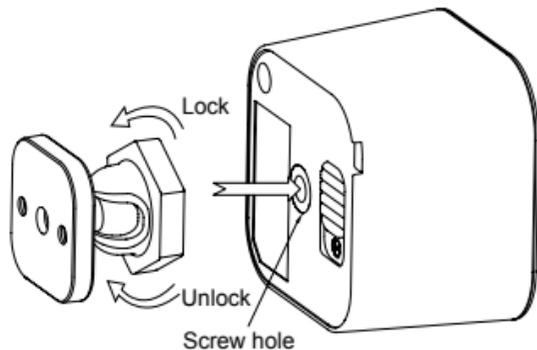
5. The Back-Mount Arm may be locked at various angles by turning the Friction Lock clockwise and counter-clockwise to respectively tighten or loosen the angle of the arm.
