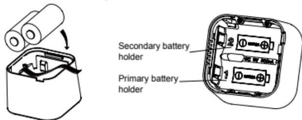
Note: If you just have only one CR123A battery, please insert the battery into the primary battery holder.
